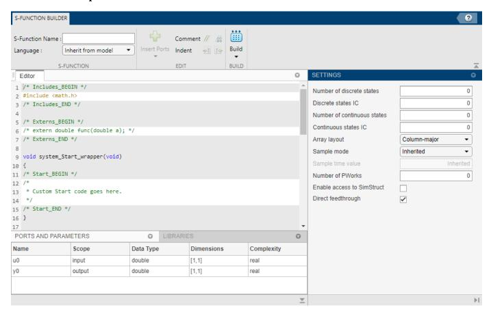
S-Function Builder editor is composed of four user interface components:
