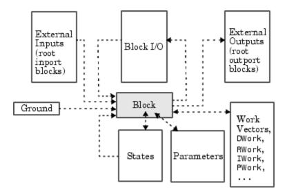
An S-function's mdlInitializeSizes routine sets the sizes of the various signals and vectors. S-function methods called during the simulation loop can determine the sizes and values of the signals.
