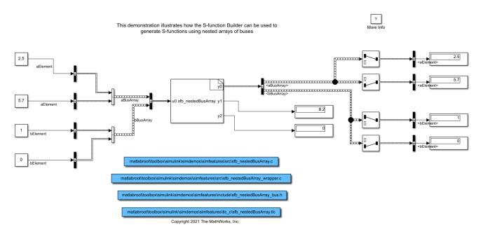
In the C code in S-Function builder, the output y0 is the nested array of buses. The output y1 is the sum of the elements of the first array of buses, aBusArray. The elements of aBusArray are aBusArray[0].aElement and aBusArray[1].aElement. The output y2 is the product of the elements of the second array of buses, bBusArray. The elements of bBusArray are bBusArray[0].bElement and bBusArray[1].bElement.
