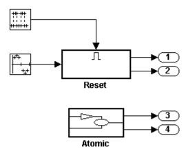
The model contains two nonvirtual subsystems, the conditionally executed enabled subsystem named Reset and the atomic subsystem named Atomic. Each subsystem contains an S-Function block that calls the S-function <code>dsfunc.c</code>, which models a discrete state-space system with two states. The enabled subsystem Reset resets the state values when the subsystem is enabled, and the output values when the subsystem is disabled.
