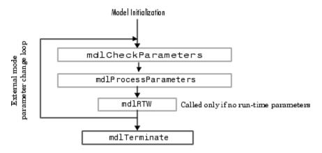
The engine calls mdlRTW once when it enters external mode and again each time a parameter changes or when you click **Update Model** on the **Modeling** tab.
